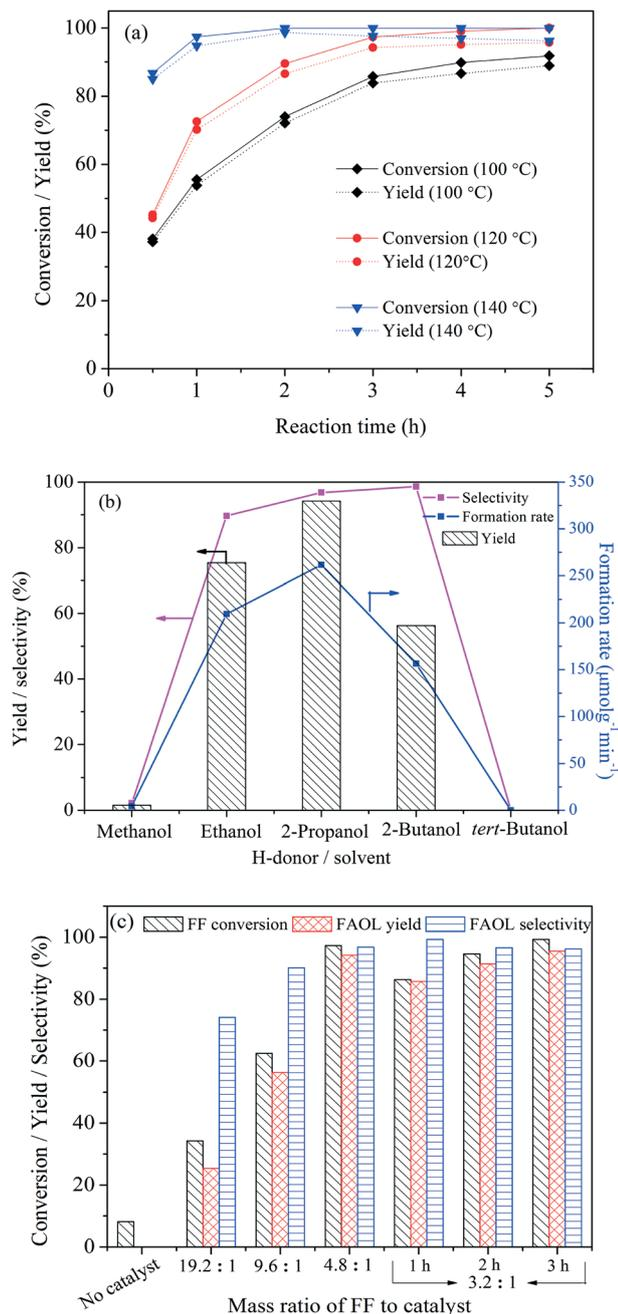
**Fig. 4** (a) Effect of reaction temperature and reaction time on CTH of FF to FAOL (1 mmol FF, 0.02 g NiO(P)-300, 5 mL 2-propanol); (b) effect of alcohol as H-donor on CTH of FF to FAOL (1 mmol FF, 0.02 g NiO(P)-300, 5 mL alcohol, 120 °C, 3 h, formation rate calculated from the FAOL yield obtained after 3 h); (c) effect of catalyst dosage on the CTH of FF to FAOL (1 mmol FF, 5 mL 2-propanol, 120 °C, 3 h, mass ratio of FF to catalyst ranging from 19.2 to 3.2).
