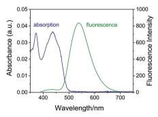
Fig. 1 UV-vis absorption and fluorescence spectra of  ${\bf 3z}$  (4  $\mu mol~L^{-1})$  in  $CH_2Cl_2.$
