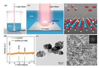
Fig. 1 Synthesis and characterization of L-CoOOH. (a) Schematic illustration of the synthesis of L-CoOOH via LAL and (b) the corresponding magnification of the laser irradiation region. (c) Schematic representation of L-CoOOH with abundant oxygen vacancies for the OER. Color code: white for H, red for O, cyan for Co, and transparent color for vacancy. (d) XRD pattern of L-CoOOH. (e and f) Low-magnification TEM and HRTEM images of L-CoOOH. The inset in (f) shows the SAED pattern of L-CoOOH.
