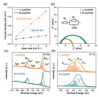
Fig. 3 Origin of the excellent OER activity of L-CoOOH. (a) The relationship between the current density and the scan rate. (b) The EIS of L-CoOOH and B-CoOOH recorded at a potential of 1.56 V<sub>RHF</sub>. (c) Co 2p and (d) O 1s XPS spectra of L-CoOOH and B-CoOOH.
