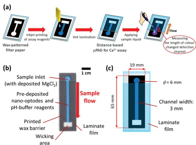
**Fig. 1** (a) Schematic procedure of device fabrication by printing technology and  $\text{Ca}^{2+}$  assay with a  $\text{Ca}^{2+}$ -selective distance-based  $\mu\text{PAD}$ ; (b) design of distance-based  $\mu\text{PAD}$  for nano-optode based  $\text{Ca}^{2+}$  detection, and (c) corresponding dimensions representing the settings in the PowerPoint graphic software.
