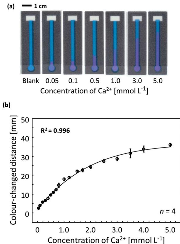
**Fig. 3** (a) Scanned images of colour-developed  $\mu$ PADs after application of the corresponding  $\text{Ca}^{2+}$  solutions of various concentrations (30  $\mu\text{L}$  of aqueous  $\text{CaCl}_2$ ); (b) software-assisted response curve of a  $\mu$ PAD-based  $\text{Ca}^{2+}$  assay; the response curve represented by the solid line was obtained with a non-linear curve fit:  $y = -124 + \frac{165}{1 + \exp\left(-\frac{x - 2.21}{1.99}\right)}$ ;
