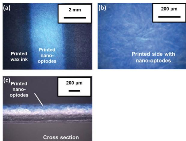
**Fig. 2** Microscope images of nano-optode filter paper substrates: (a) nano-optode modified paper surface of the flow channel; (b) scale-up of the nano-optode modified paper surface; and (c) cross section of nano-optode modified paper.
