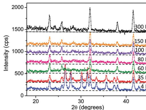
Fig. 7 Neutron diffraction data collected for  $\text{Ca}_2\text{Mn}_3\text{O}_8$  showing the temperature dependence of the deviations/Warren-like behaviour of the background. Note the dotted line is a guide for the eye.
