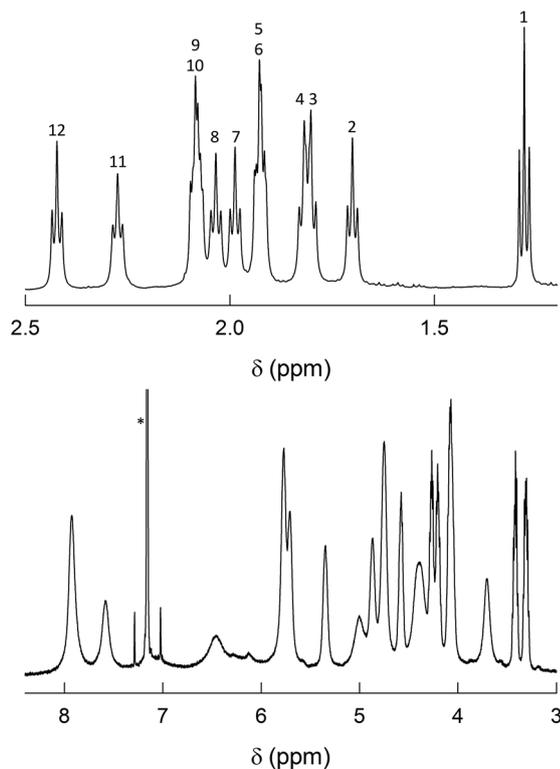
Fig. 3  $^1\text{H}$  NMR spectrum of 1 mM  $\text{Au}_{144}(\text{SC}_2)_{60}$  in  $\text{C}_6\text{D}_6$  at 25  $^\circ\text{C}$ . For convenience, the spectrum has been divided into two parts:  $\beta\text{-CH}_3$  (top) and  $\alpha\text{-CH}_2$  (bottom). In the latter, the scale has been enlarged (9.3 $\times$ ). The numbers on the top plot label the 12 ligand types (cf. Fig. S4 $\dagger$ ). The asterisk marks the benzene signal.
