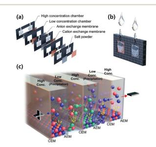
Fig. 1 (a) Layered structure of the ssRED consisted of alternating HC and LC chambers. The outermost membranes constitute the interface with the target devices. (b) Schematic diagram of ssRED activation. Entry of water through inlets and dissolution of solid salts in high concentration chambers activate the ssRED. (c) Working principles of PssRED operation.
