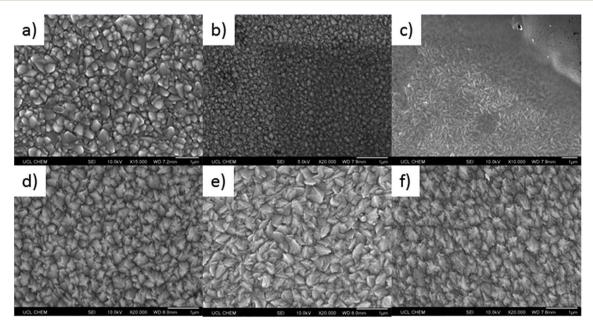
Fig. 3 Typical SEM images showing the surface morphology for (a) undoped SnO<sub>2</sub>, (b) 0.1 mol% P:SnO<sub>2</sub>, (c) 0.25 mol% P:SnO<sub>2</sub>, (d) 0.5 mol% P:SnO<sub>2</sub>, (e) 1.0 mol% P:SO<sub>2</sub>, and (f) 1.5 mol% P:SnO<sub>2</sub> thin films on glass. All samples were produced at 550 °C, by aerosol assisted CVD using compressed air as the carrier gas.
