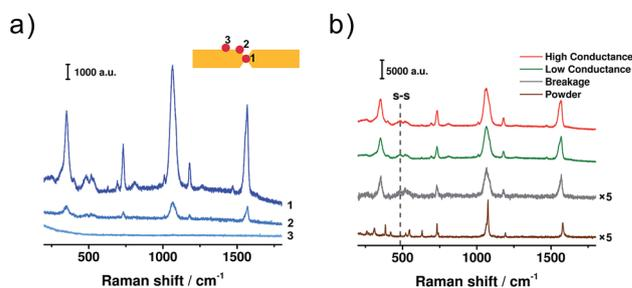
Fig. 3 (a) SERS spectra of **BDT** collected from different sites of the electrode pair. Inset: the locations of the laser spot. (b) SERS spectra collected when the molecular junction was mechanically controlled at the regimes of high conductance (red), low conductance (green), and breakage (grey), respectively. An ordinary Raman spectrum of **BDT** powder (brown) is displayed for comparison. Laser excitation: 785 nm.
