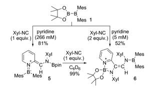
Scheme 3 Reaction of 1 with Xyl-NC in the presence of an excess of pyridine (yields estimated by  $^1$ H NMR spectroscopy. The concentration of 1 or 5 is given in parentheses below pyridine).
