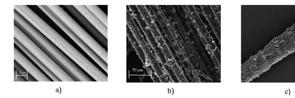
Fig. 4 (a) SEM image of untreated glass fibre roving ( $\times$ 2000); (b) SEM image graphene-based (coated) glass roving ( $\times$ 500); and (c) SEM image graphene-based (coated) glass roving ( $\times$ 1000).
