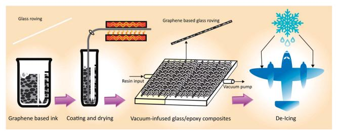
Fig. 1 Process flow diagram for manufacturing graphene-based glass/epoxy composites for de-icing applications.
