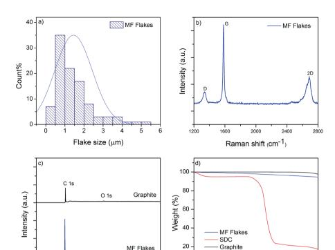
Fig. 2 (a) The size distribution of MF flakes; (b) Raman spectra of MF flakes; (c) wide scan XPS spectra of starting graphite and MF flakes; (d) TGA curves of MF flakes, SDC and Graphite.
