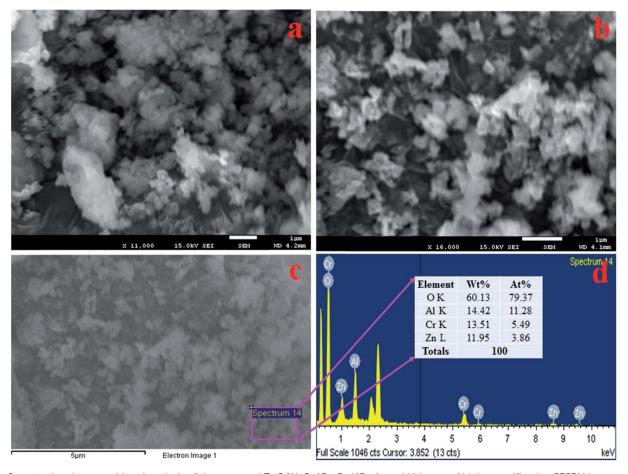
Fig. 3 Structural and compositional analysis of the prepared ZnO/Al<sub>2</sub>O<sub>3</sub>/Cr<sub>2</sub>O<sub>3</sub> NPs. (a and b) Low and high magnification FESEM images and (c and d) elemental analysis with EDS
