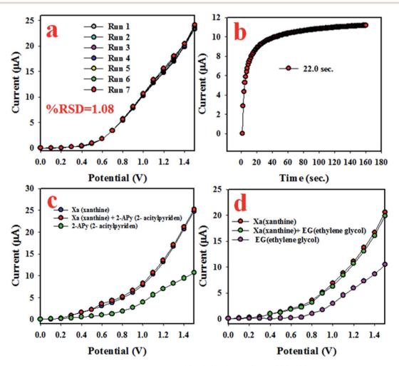
Fig. 5 Reliability investigations of the XNT sensor based on ZnO/Al<sub>2</sub>O<sub>3</sub>/Cr<sub>2</sub>O<sub>3</sub> NPs/binder/GCE: (a) testing reproducible performance, (b) response time, and (c and d) interference tests.
