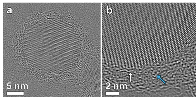
**Fig. 4** A focal series of 15 HRTEM images are used to perform exit wave reconstruction. Phase images of the reconstructed exit wave of different particles show clearly the presence and position of the polymer shell around the particles. The white arrow indicates the presence of parallel oriented polymer chains, while the blue arrow shows the presence of chains in different orientations.
