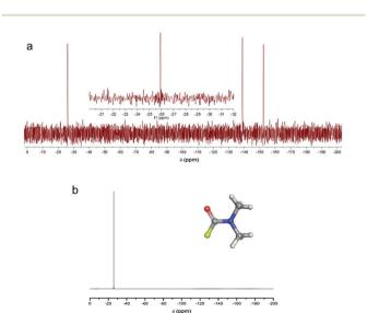
Fig. 8 (a) <sup>19</sup>F NMR spectrum (in DMF, 470 MHz) of the supernatant liquid obtained from a FG/DMF suspension heated at 120 °C for 5 hours and stirred at room temperature overnight (in the inset, a close-up of the peak at -26 ppm is shown). (b) <sup>19</sup>F NMR spectrum (in DMF, 470 MHz) of the separately prepared compound F-DMF (structure shown in inset). (b) <sup>19</sup>F NMR spectrum (in DMF, 470 MHz) of the separately prepared compound F-DMF (structure shown in inset).
