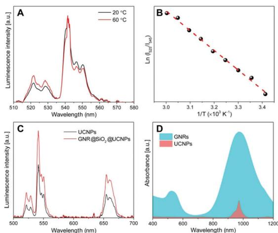
**Fig. 3** (A) Normalized upconversion luminescence spectra of UCNP at two different temperatures. (B) The temperature dependence of the ratio calculated from the luminescence spectra obtained at various temperatures. Dots are experimental results and the red line is the best linear fit. (C) Upconversion luminescence spectra of UCNP and GNR@SiO<sub>2</sub>@UCNP. (D) Normalized absorption spectra of UCNP and GNRs.
