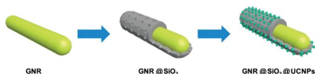
**Scheme 1** Schematic illustration of the synthetic procedure for the preparation of the GNR@SiO<sub>2</sub>@UCNPs nanocomposite.
