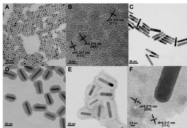
**Fig. 1** (A) TEM and (B) HR-TEM images of the synthesized NaGdF<sub>4</sub>:Er<sup>3+</sup>, Yb<sup>3+</sup> UCNPs. TEM images of the (C) synthesized GNRs, (D) the SiO<sub>2</sub> coated GNRs (GNR@SiO<sub>2</sub>), and (E) the hybrid SiO<sub>2</sub> coated GNRs decorated with NaGdF<sub>4</sub>:Er<sup>3+</sup>, Yb<sup>3+</sup> UCNPs (GNR@SiO<sub>2</sub>@UCNPs), (F) HR-TEM image of the GNR@SiO<sub>2</sub>@UCNPs interface.
