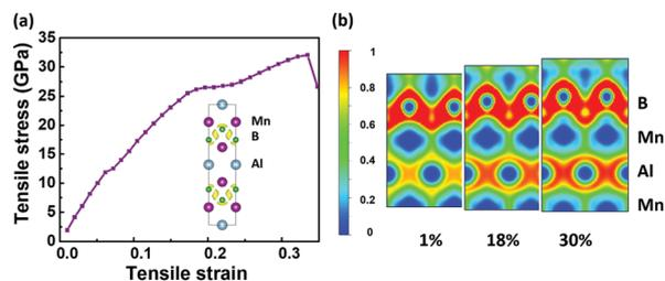
**Fig. 2** (a) The calculated stress–strain curve of  $\text{Mn}_2\text{AlB}_2$  with the ELF contour plots and (b) projected on the plane containing Mn and Al atoms under  $[0001]$  tensile strains of 1%, 18%, and 30%.
