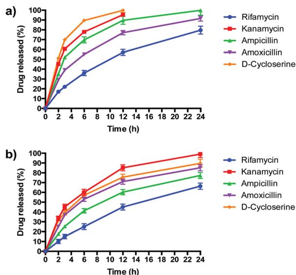
Fig. 5 The release profiles of antibiotics from PLGA nanoparticles and PLGA/DOTAP nanoparticles. *In vitro* release profiles of different antibiotics from (a) PLGA nanoparticles and (b) PLGA/DOTAP nanoparticles in PBS (pH 7.4) for 24 h at 37 °C ( $n = 5$ , mean  $\pm$  S.D.).
