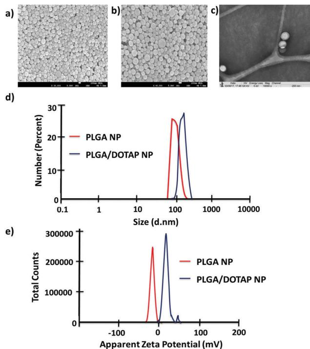
**Fig. 1** Physicochemical properties of PLGA nanoparticles and PLGA/DOTAP nanoparticles. SEM images of (a) PLGA nanoparticles and (b) PLGA/DOTAP nanoparticles. (c) TEM image of PLGA/DOTAP nanoparticles. (d) Dynamic laser scattering of PLGA nanoparticles and PLGA/DOTAP nanoparticles. (e) Zeta potential of PLGA nanoparticles and PLGA/DOTAP nanoparticles.
