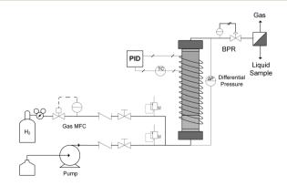
Fig. 1 Reactor Schematic Diagram.  $\mu PBR$  with gas (MFC) and liquid (pump) flow control differential pressure measurement, back pressure regulation (BPR), temperature control (PID) and post-reaction effluent fractionation.
