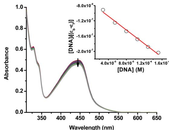
Fig. 4 UV-vis spectra of compound **3** (50% DMSO in Tris-HCl buffer at pH = 7.2) with an incrementing concentration of calf thymus DNA base pairs. The inset shows a linear fit of the first 6 data points into eqn (1) to extract the intrinsic binding constant ( $K_b$ ) of compound **3** to DNA base pairs.
