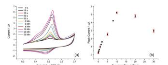
Fig. 2 Assessment of electrode exposure times to 1.0  $\mu$ M Hg<sup>2+</sup> by CV. (a) Voltammograms of AuNP@TA-GCE at various exposure times. (b) Current behaviour at peak-2 at exposures ranging from zero to 30 minutes.
