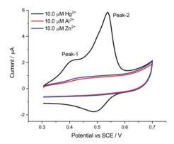
Fig. 4 Selectivity performance of the AuNP@TA-GCE for  $Al^{3+}$  and  $Zn^{2+}$  at a scan rate of  $0.1 \text{ V s}^{-1}$  and exposure time of 10 min.
