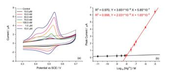
Fig. 3 Detection of Hg<sup>2+</sup> by CV. (a) Voltammograms of AuNP@TA-GCE at varying concentrations of Hg<sup>2+</sup>. (b) Linear peak current behaviour at various Hg<sup>2+</sup> concentrations.
