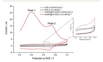
Fig. 1 Detection of  ${\rm Hg}^{2+}$  at an unmodified GCE, as well as at a functionalized AuNP@TA-GCE at a scan rate of 0.1 V s<sup>-1</sup>.
