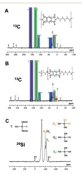
Fig. 8 Solid-state MAS NMR spectra. Spinning side-bands are labelled with \*. (A) <sup>13</sup>C spectrum of PI6 after sintering. (B) <sup>13</sup>C spectrum of PI6/ SiO<sub>2</sub> after sintering. (C) <sup>29</sup>Si spectrum of PI6/SiO<sub>2</sub> after sintering
