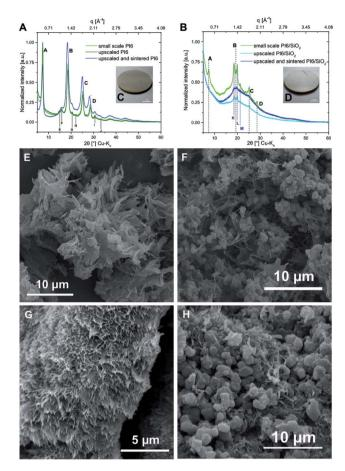
Fig. 7 PI6 and PI6/SiO<sub>2</sub> upscaling and sintering. (A) and (B) Comparison of the diffractograms of small scale synthesis, upscaled synthesis and material after sintering (PI6: (A) PI6/SiO<sub>2</sub>: (B)). (C) and (D) Photographs of the PI6 (C), and the PI6/SiO<sub>2</sub> pellet from sintering. (E)-(H) SEM images of upscaled PI6 before (E) and after (G) sintering, and of upscaled PI6/SiO<sub>2</sub> before (F) and after (H) sintering.
