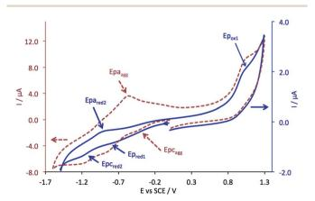
Fig. 3 CV of 5, on Pt disc electrode, in DMF containing 0.1 M  $Bu_4 NPF_6$ , at a scan rate of 0.1 V s $^{-1}$ , at a concentration of  $10^{-3}$  mol  $L^{-1}$  (solid blue line) and at  $4\times10^{-3}$  mol  $L^{-1}$  (aggregation, dashed red line).
