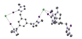
Fig. 3 One section of the crystal packing of  $[1-l](BF_4)$ . Solvent  $(CHCl_3)$ ,  $BF_4^-$  anions and hydrogen atoms have been omitted for clarity. The crystal packing is showing the halogen bonding interaction between the jodo atoms from two molecules with the chloride.
