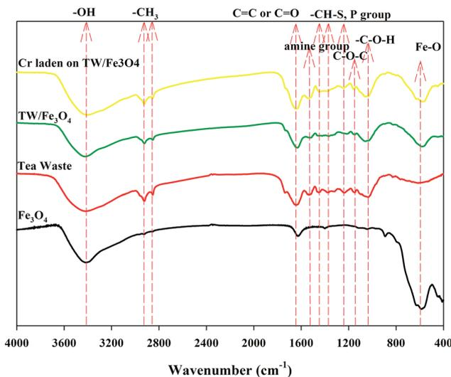
Fig. 4 The FTIR spectrum of tea waste, Fe<sub>3</sub>O<sub>4</sub>, TW/Fe<sub>3</sub>O<sub>4</sub> and Cr laden on the TW/Fe<sub>3</sub>O<sub>4</sub> composite.
