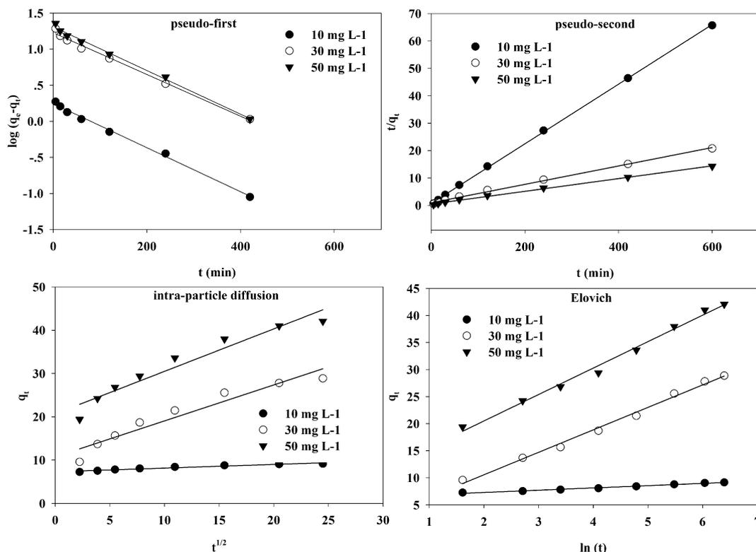
Fig. 8 Pseudo-first-order, pseudo-second-order, intra-particle diffusion, and Elovich kinetics models of Cr(vi) adsorption onto the TW/Fe<sub>3</sub>O<sub>4</sub> composite at 298 K.
