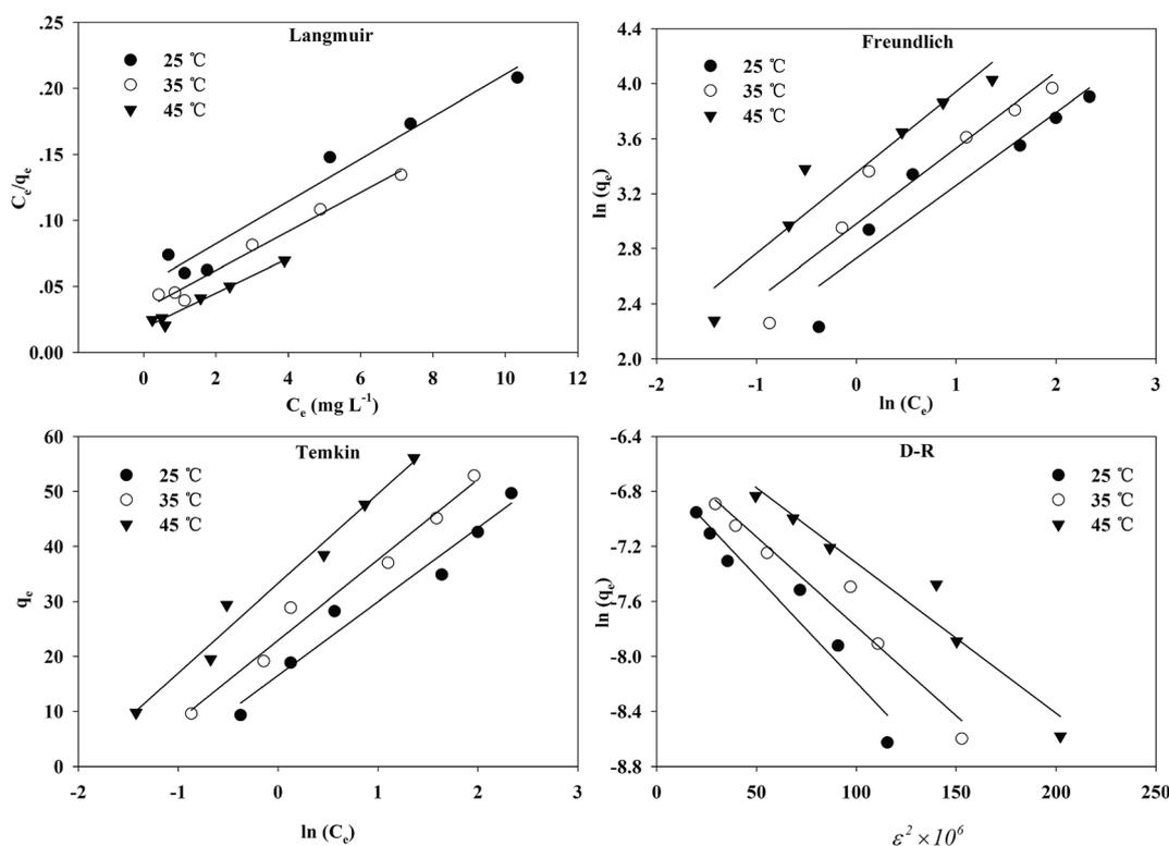
Fig. 9 The fitting of Langmuir, Freundlich, Temkin, D–R isotherms for Cr(vi) adsorption onto the TW/Fe<sub>3</sub>O<sub>4</sub> composite.
