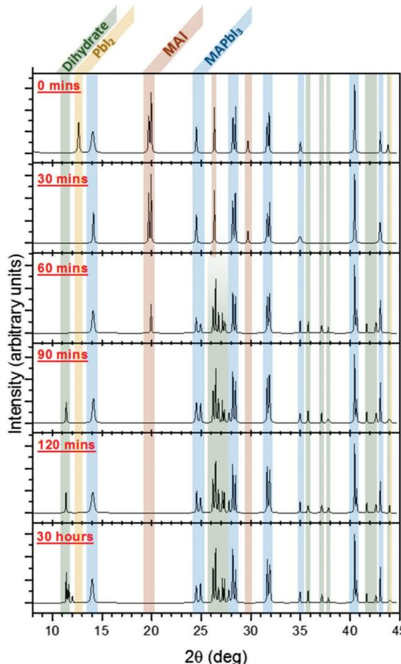
Fig. 8 X-ray diffraction patterns following the evolution of  $\text{MAPbI}_3$  from the initial bilayer MAI/ $\text{PbI}_2$  films (0 min), to the nascent perovskite (30 min), and then finally to the  $\text{MAPbI}_3$  film (90 min). After 90 min, the dihydrate  $\text{MA}_4\text{PbI}_6 \cdot 2\text{H}_2\text{O}$  is observed to form ( $2\theta = 11.4^\circ, 11.5^\circ, \text{ and } 11.6^\circ$ ). Reproduced from ref. 78, Copyright 2015, American Chemical Society.
