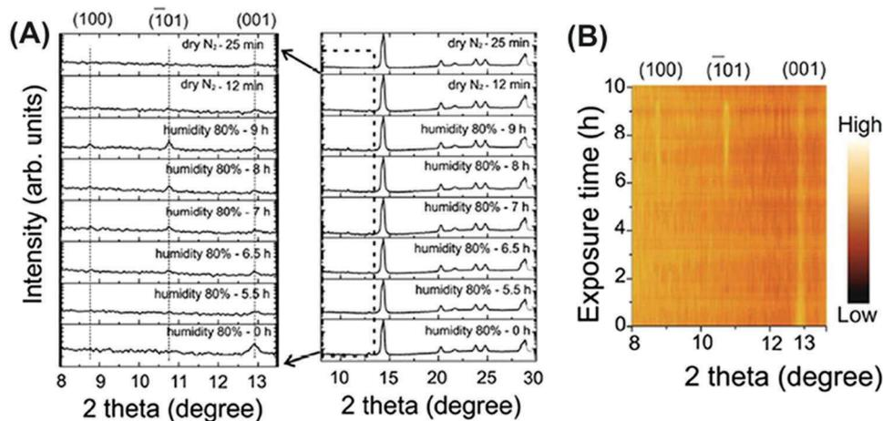
Fig. 10 (A) Time-resolved *in situ* XRD of a MAPbI<sub>3</sub> film during the first hydration–dehydration round and a zoomed-in image at  $2\theta$  angles from  $8.0^\circ$  to  $13.5^\circ$ . (B) The corresponding contour plot showing changes in XRD peak intensity during the first hydration–dehydration cycle. Reproduced from ref. 93, Copyright 2016 American Chemical Society.
