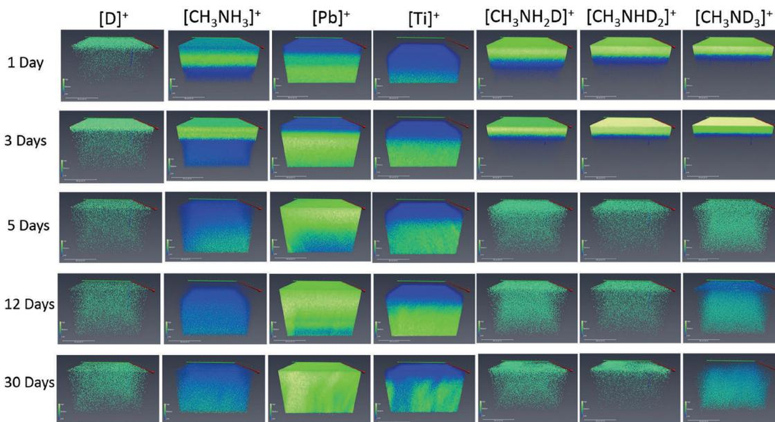
Fig. 9 3D reconstructed images of deuterium, methylammonia, PbI<sub>2</sub>, and TiO<sub>2</sub> at different exposure times. Color map illustrating the molecular density from high (bright green) to low (blue). Reproduced from ref. 92, Copyright 2017 Wiley-VCH Verlag GmbH & Co. KGaA.
