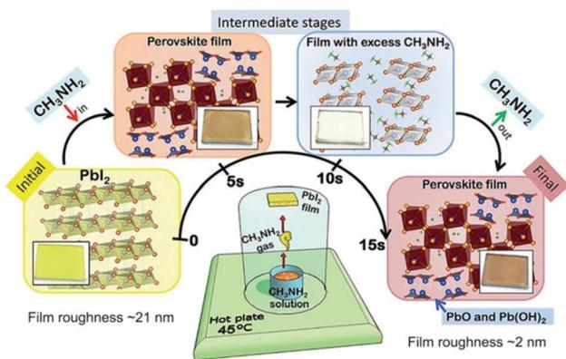
Fig. 7 Methylamine gas induced perovskite formation. Illustration of the setup used for processing perovskite at room temperature from simple precursors of  $\text{CH}_3\text{NH}_2$  gas; the  $\text{PbI}_2$  film is depicted in the lower middle part of the figure. Reproduced from ref. 77 with permission from The Royal Society of Chemistry.
