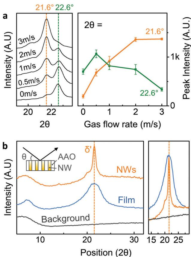
Fig. 2 (a) (left) XRD patterns of nanowire-filled templates crystallised at various assisted gas-flow rates. (right) Based on the normalised XRD patterns, the average intensity of the peak at  $21.6^\circ$  and  $22.6^\circ$  is plotted as a function of assisted-gas flow rate. (b) XRD patterns of a nanowire-filled template (orange), melt-quenched film (blue), and silicon background (grey). The right image shows the magnification of the  $\delta'$ -phase range.
