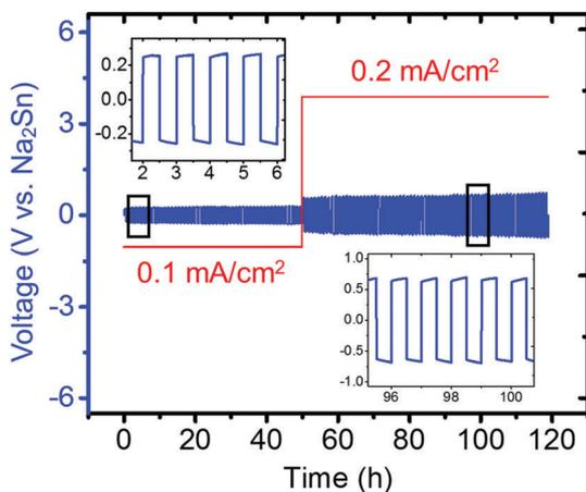
Fig. 10 Electrochemical cycling of Na<sub>2</sub>Sn|Na<sub>3</sub>PS<sub>4</sub>|Na<sub>2</sub>Sn symmetric cell (60 min per charge and discharge). The insets present zoomed-in voltage profiles during cycling from 2–6 h and 96–100 h.
