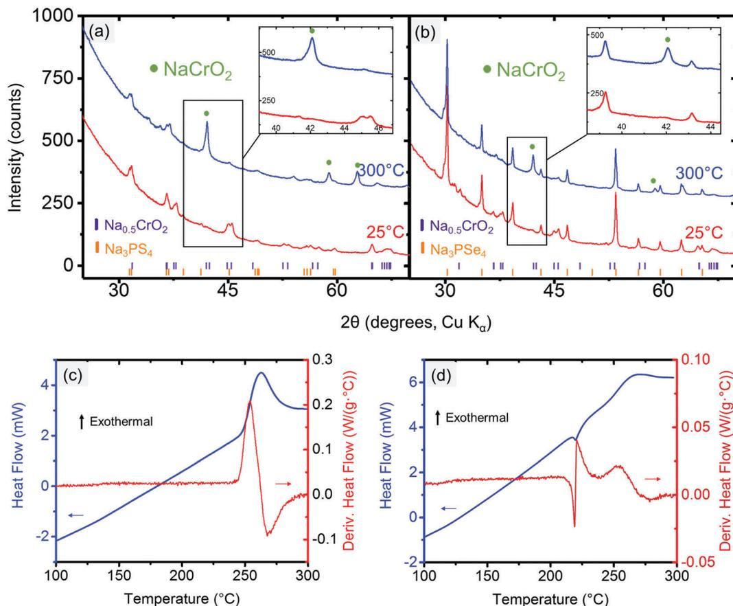
Fig. 6 XRD results for reaction between (a)  $\text{Na}_{0.5}\text{CrO}_2$  and  $\text{Na}_3\text{PS}_4$  and (b)  $\text{Na}_{0.5}\text{CrO}_2$  and  $\text{Na}_3\text{PSe}_4$  at RT (25 °C) and 300 °C. DSC results for reaction between (c)  $\text{Na}_{0.5}\text{CrO}_2$  and  $\text{Na}_3\text{PS}_4$  and (d)  $\text{Na}_{0.5}\text{CrO}_2$  and  $\text{Na}_3\text{PSe}_4$ .
