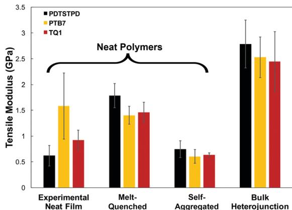
Fig. 11 Summary of tensile modulus predictions and comparison to experiment.
