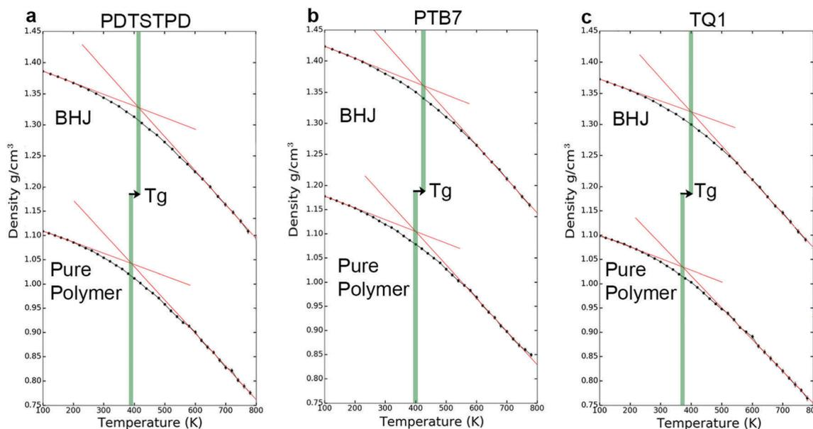
Fig. 5 Thermal properties, density vs. temperature curves showing glass-transitions of polymer: PC<sub>71</sub>BM bulk heterojunctions (top curves) and pure polymers (bottom curves) for (a) PDTSTPD, (b) PTB7, and (c) TQ1.
