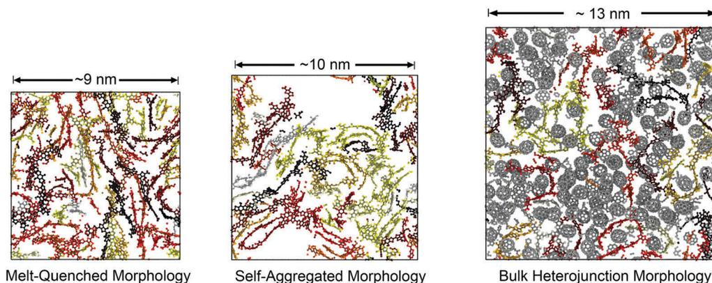
Fig. 8 Comparison of the three glassy, solid morphologies ( $T = 300$  K and  $p = 1$  atm) for PTB7. Snapshots showing 2 nm slices of the simulation trajectory. Polymers are coloured separately. Hydrogen atoms and side chains are omitted for clarity.
