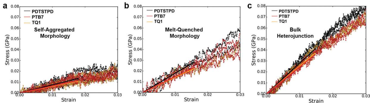
Fig. 10 Mechanical response. Stress–strain curves showing the responses of (a) the self-aggregated morphology, (b) the melt-quenched morphology, and (c) the bulk heterojunction morphology of each polymer. The solid lines overlaid on the plots are the linear fits used to calculate the tensile moduli. It can be seen in the plots that different morphologies and compositions play a more important role in determining the stress response than differences in molecular structure.
