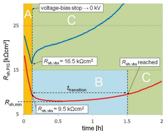
Fig. 28  $R_{sh}$  measurements (normalized) of two one-cell modules during degradation and regeneration. One module exhibits the transition phase (marked by red) whereas the other module does not (marked by blue). The shunting phase (A), the transition phase (B) and the regeneration phase (C) are shown using different colours. The initial  $R_{sh}$  value (normalized) of both modules is more than 1 MΩ cm<sup>2</sup>, which is not shown in the figure. Reprint from ref. 62. Copyright 2013, WIP.
