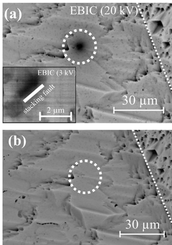
**Fig. 25** EBIC measurements (20 kV) at a PID shunt location before (a) and after (b) a thermal recovery process. The PID-s disappeared after recovery. The inset in (a) shows the PID-s defect before recovery at a low electron acceleration voltage (3 kV) and hence with an increased lateral resolution. The dotted line represents a grain boundary as guide to the eyes. Reprint from ref. 72. Copyright 2014, Elsevier.
