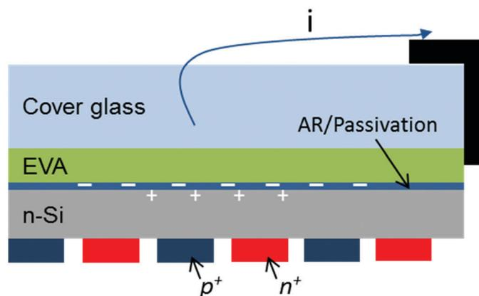
**Fig. 10** A schematic diagram illustrating the surface polarization effect in SunPower's n-type high-efficiency back-contact c-Si cells. EVA is used as the encapsulant foil. "i" represents the leakage current from cell through glass to frame and earth ground. Adapted from ref. 27.
