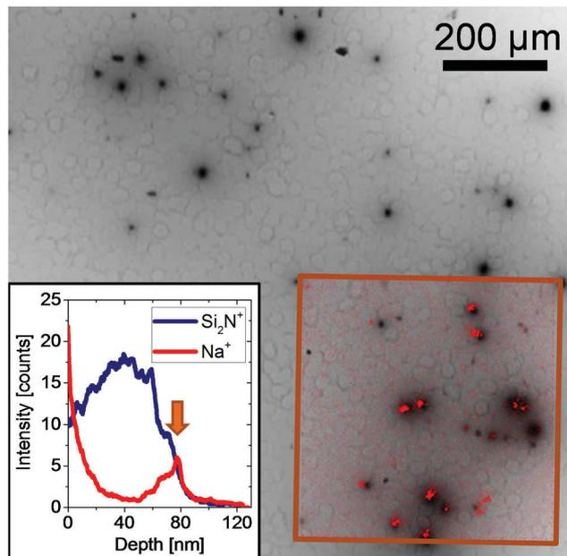
Fig. 4 An EBIC image of a monocrystalline silicon cell region with a high density of PID shunts acquired at an acceleration voltage of 30 kV. The inset shows the distribution of Na at the  $\text{SiN}_x/\text{Si}$  interface measured by the ToF-SIMS. Reprint from ref. 65. Copyright 2014, Elsevier.
