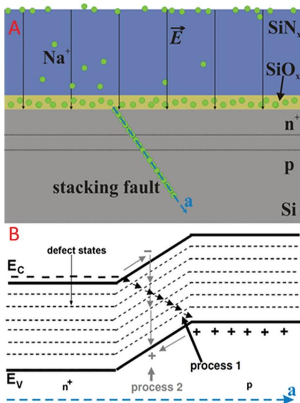
Fig. 6 (A) Schematic drawing of a solar cell cross section and transport of  $\text{Na}^+$  (green dots) through the  $\text{SiN}_x$  layer and subsequent diffusion into the stacking faults. (B) The proposed band structure along a Na decorated stacking fault. Reprint from ref. 65. Copyright 2014, Elsevier.
