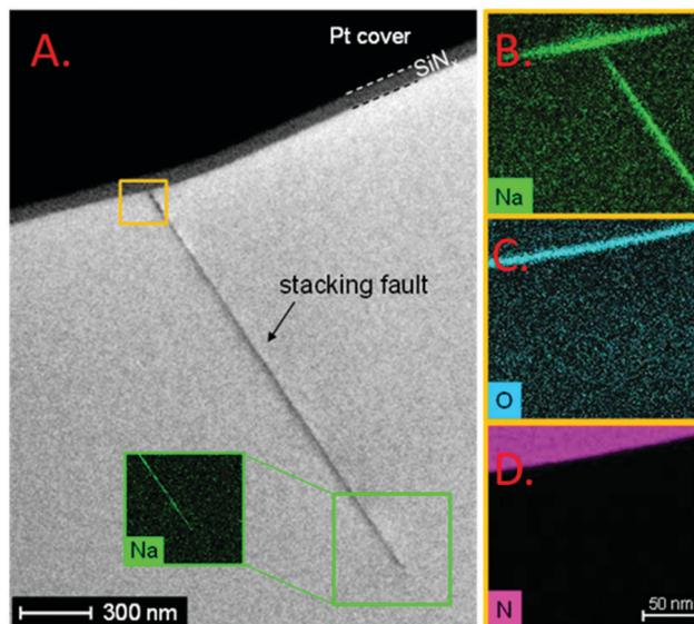
Fig. 5 (A) A bright-field TEM image of a stacking fault representing a single PID-shunt. (B–D) EDX mappings acquired in the STEM mode at the same stacking fault near the interface between Si and  $\text{SiN}_x$ . A Na-EDX map of the lower part of the stacking fault is also shown in the inset of A. Reprint from ref. 65. Copyright 2014, Elsevier.
