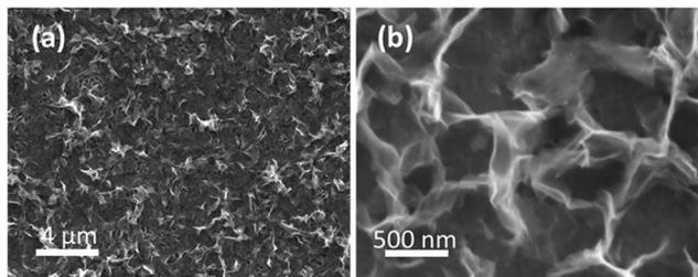
Fig. 6 SEM images of electrodeposited  $\text{Co(OH)}_2$  on the Au electrode after the OER performed for 5 cycles under the conditions of Fig. 5.
