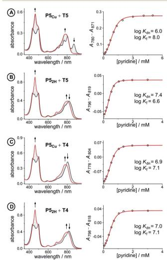
Fig. 5 UV-vis-NIR denaturation titrations of linear porphyrin oligomer complexes with templates T4 and T5 (all in CHCl3 at 298 K). The spectra shown on the left are those of the 1:1 complexes (black) and the end spectra of the pyridine-saturated oligomers (red). On the right the experimental (black circles) and calculated binding isotherms (red lines) are shown. All titrations were performed at least twice (see ESI, Section S1.2†).
