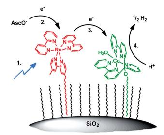
Scheme 4 Proposed reaction mechanism of photocatalytic H<sub>2</sub> production on hydrophobic silica: (1) photoexcitation of  $5 \rightarrow 5^*$ ; (2) reductive quenching of  $5^* \rightarrow 5^-$ ; (3) electron transfer  $5^- \rightarrow 3$ ; (4) H<sup>+</sup> reduction by 3-
