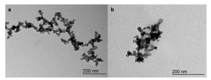
Fig. 1 Representative TEM micrograph of hydrophilic fumed silica without (a) and hydrophobic fumed silica with adsorbed PS 5 from a diluted aqueous suspension with 7 as surfactant (b).
