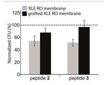
Fig. 5 Antimicrobial effect of peptides bonded to the membranes: *E. coli* colony forming units (CFU) after 30 min exposure, as percentage of CFU on unmodified membranes controls. Two types of control membranes are used and indicated with the dashed line: commercial XLE membrane (control for gray bars), or the copolymer coated XLE membrane surface (control for the black bars). Average of 3 independent experiments including the standard deviation is shown.
