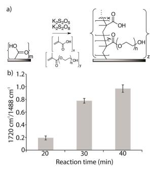
Fig. 2 (a) LE 440 RO membrane surfaces were modified with a copolymer of methacrylic acid and poly(ethylene glycol)methacrylate. (b) FTIR absorbance ratio 1720  $\rm cm^{-1}/1488~cm^{-1}$  of modified surfaces at different reaction times, at 25 °C.
