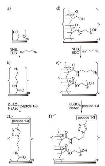
Fig. 3 Attachment of antimicrobial peptides to LE 440 RO membrane surfaces: for non-grafted membrane surface (a): attachment of azide functionality (b); and immobilization of peptide using click chemistry (c). For membrane surface grafted with copolymer of methacrylic acid and poly(ethylene glycol)methacrylate (d): attachment of azide functionality to grafted surface (e); immobilization of peptide on grafted surface using click chemistry (f).
