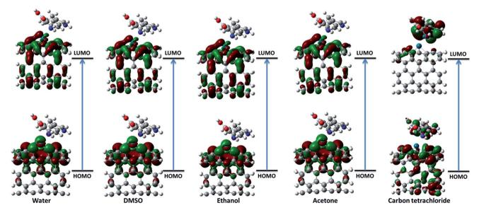
Fig. 2 The distribution of HOMO and LUMO orbitals of complex 1 in different solvents.
