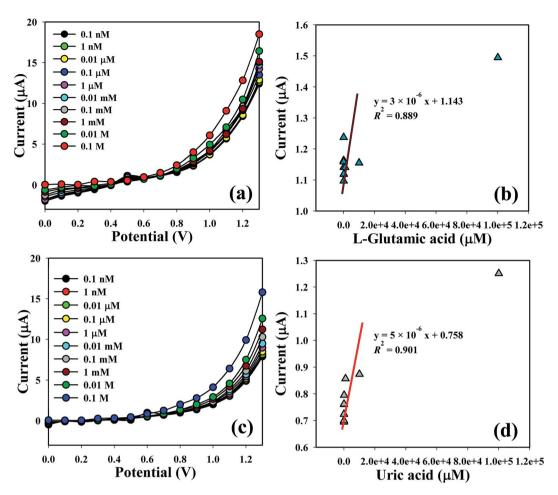
Fig. 6  $Co_3O_4$  NSs coated GCE for sensing by I-V response with (a and c) concentration variation; (b and d) are the calibration curves of L-GA and UA, respectively
