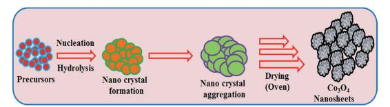
Scheme 2 Growth mechanism of mesoporous Co<sub>3</sub>O<sub>4</sub> nanosheets.
