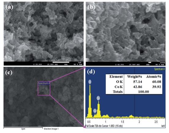
Fig. 2 (a and b) Low and high magnified images and (c and d) elemental analysis of the Co<sub>3</sub>O<sub>4</sub> NSs
