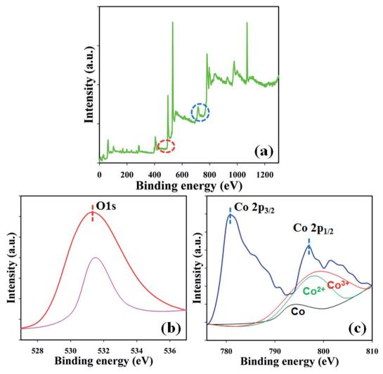
Fig. 3 Binding energy analysis (a) full spectrum, (b) O 1s, and (c) spin orbit Co 2p level of the NSs.
