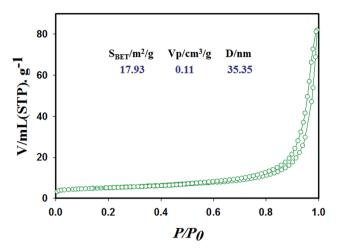
Fig. 4 Surface characterization of the cobalt oxide nanosheets material with specific surface area, pore volume and pore size by N<sub>2</sub> adsorption-desorption isotherms.
