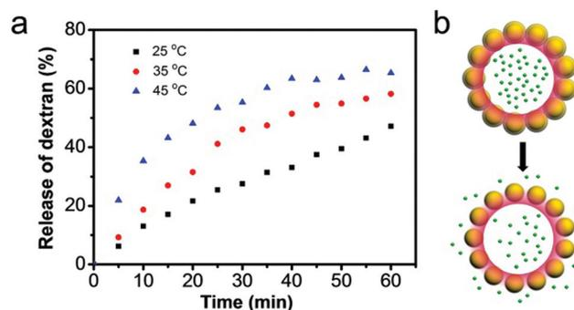
**Fig. 7** (a) The release profiles of 150 kDa FD cargo from microcapsules over 1 h, at temperatures: 25, 35 and 45 °C. (b) Schematic representation of the contraction of the colloidal particles upon increasing temperature, resulting in release of encapsulated cargo.
