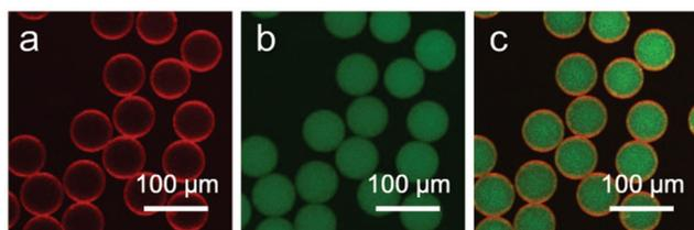
**Fig. 5** CLSM images of microdroplets encapsulating fluorescein isothiocyanate-dextran cargo and capsule-forming components: MCP, AP and CB[8]. (a) Red channel: Rhodamine B-labelled AP, (b) green channel: FD and (c) overlaid.
