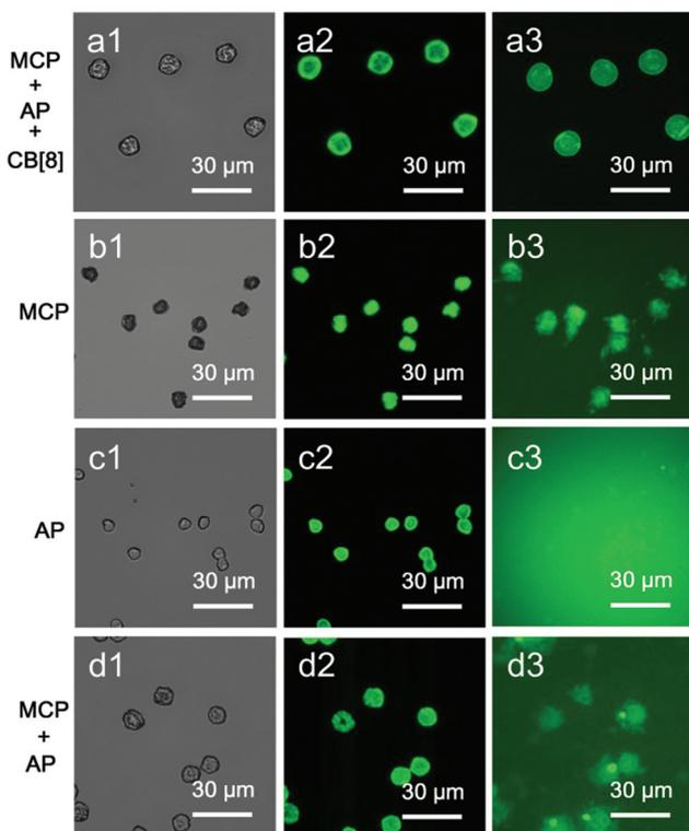
**Fig. 6** (a1) Optical and (a2) fluorescence micrographs of dried supramolecular microcapsules loaded with FD (150 kDa), and (a3) after rehydration in water for 5 minutes. This is compared with microstructures prepared from microdroplets containing (b1–b3) only the MCP component, (c1–c3) only AP component, and (d1–d3) MCP and AP components in the absence of CB[8].
