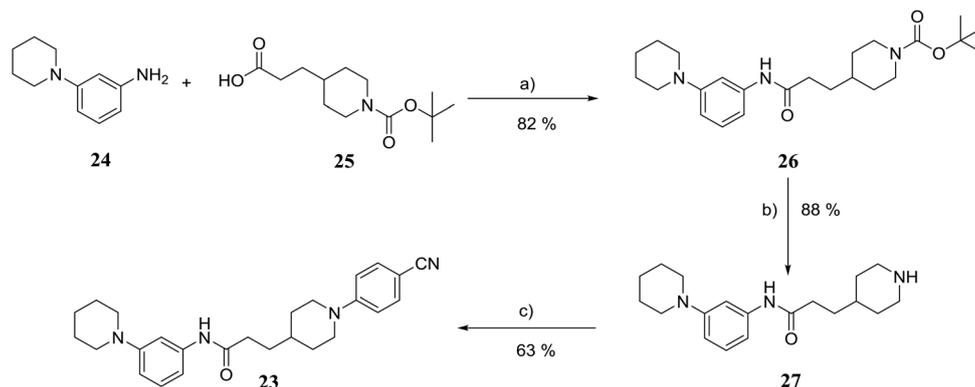
**Fig. 8** Synthetic scheme for the preparation of 3-(1-(4-cyanophenyl)piperidin-4-yl)-*N*-(3-(piperidin-1-yl)phenyl)propanamide (**23**). (a) DCM, DIPEA, COMU, 22 °C; (b) TFA, DCM, 22 °C; 2 h; (c) 4-fluorobenzonitrile, K<sub>2</sub>CO<sub>3</sub>, anhydrous DMSO, 100 °C; 3 h.
