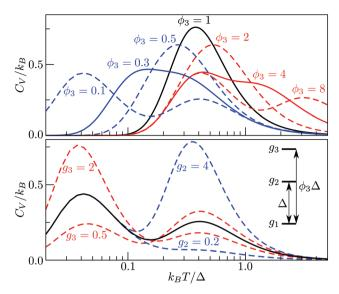
Fig. 2 Heat capacity of a three-level system with different values of  $g_2$ ,  $g_3$  and  $\phi_3$ , with  $\Delta$  (i.e. the energy gap between the ground state and the first excited state) setting the energy scale. The default values are  $g_1$  =  $g_2 = g_3 = 1$  and  $\phi_3 = 0.1$ . Note the logarithmic scale on the horizontal axis.
