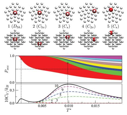
Fig. 7 Occupation probabilities, stacked and colour-coded as in Fig. 3, and (partial) heat capacity plots focusing on the low-temperature precursor anomalies in Fig. 6 for  $\sigma_r = 0.992$ . The five lowest-energy minima are shown for illustration, viewed down the principal axis (top row) and along the orthogonal plane (bottom), with the larger red sphere representing the dopant.
