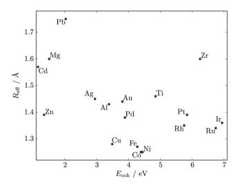
Fig. 10 Scatter plot of cohesive energy  $E_{coh}$  (per atom) and effective atomic radius  $R_{\rm eff}$  for various 12-coordinated (i.e. fcc or hcp) metals. <sup>26,54</sup>
