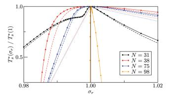
Fig. 5 Scaled  $T_s^*$  versus dopant relative size  $(\sigma_r)$  for selected LJ<sub>N</sub> clusters. Dashed and dotted curves represent data with the vibrational and landscape components of the configurational entropy, respectively, set to the values for the homoatomic cluster  $(\sigma_r = 1)$ .
