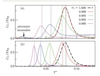
Fig. 6 Heat capacity of doped LJ $_{75}$  clusters for different values of  $\sigma_{\rm r}$ , calculated using either (a) all local minima or (b) just biminima. Dashed vertical lines mark the value of  $T_{\rm s}^*$  calculated using (7).
