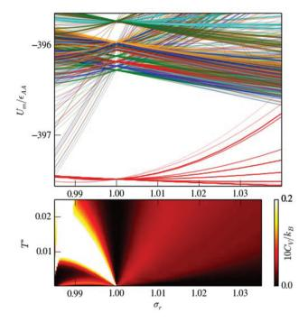
Fig. 8 The potential energy spectrum of low-lying minima (top) and low-temperature heat capacity map (bottom) for doped LJ<sub>75</sub> as a function of the dopant relative size  $\sigma_r$ . In the top diagram, energy levels emanating from the same degenerate homoatomic ( $\sigma_r = 1$ ) minima are coloured the same. The bottom diagram highlights the low-temperature ( $T^* < 0.25$ )  $C_V$  peak(s) corresponding to permutational isomerisation.
