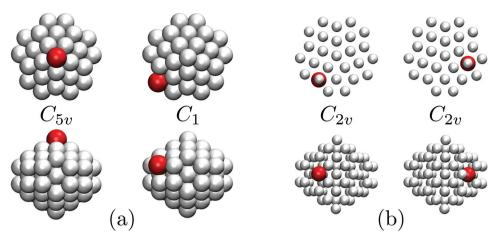
Fig. 11 The two lowest-energy minima for (a)  $Ni_{74}$ Ag and (b)  $Ni_{74}$ Pt Marks decahedra,<sup>23</sup> viewed down the principal axis (top) and along the orthogonal plane (bottom). The larger red sphere represents the dopant, and the host atom size is varied for clarity.
