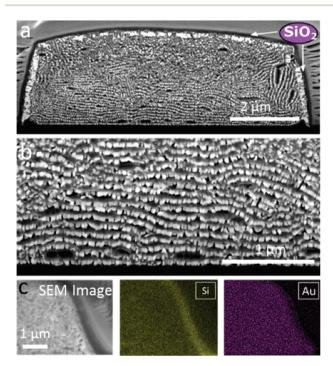
**Fig. 5** Characterization of GNR supercrystals coated with a mesoporous silica film. (a and b) SEM images of a supercrystal cross section (after the FIB process) at different magnifications. (c) EDX mapping of silicon (Si) and gold (Au) at the edge of a GNR-silica supercrystal.
