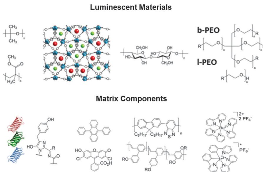
Fig. 2 Upper part – exemplary of the components used for the matrix – *i.e.*, cross-linked polymers (left), MOF (central left), cellulose (central right), and non-cross-linked branched (b-PEO) and linear (l-PEO) polyethyleneoxide derivatives (right). Lower part – exemplary of the luminescent materials – *i.e.*, fluorescent proteins (left), small-molecules (central left), polymers (central right), and coordination complexes (right).
