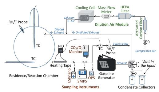
Fig. 1 Simplified schematics of the environmental chamber setup. "RH/T Probe" stands for "relative humidity and temperature probe". "TC" stands for "thermocouple". "PID" stands for "proportional-integral-derivative controller". "ESPnano" is the electrostatic precipitator. "SMPS" stands for "scanning mobility particle sizer". "OPS" stands for "optical particle sizer". "HEPA filter" stands for "high efficiency particulate air filter".
