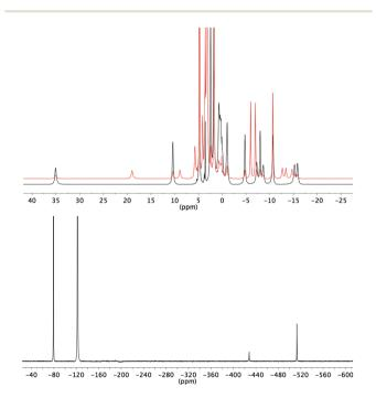
Fig. 3 NMR spectra of EuL $^3$  (D $_2$ O, 500 MHz, 278 K). Top:  $^1$ H NMR in the absence (black) and presence (red) of an excess of sodium fluoride; Bottom:  $^{19}$ F NMR in the presence of an excess of sodium fluoride.
