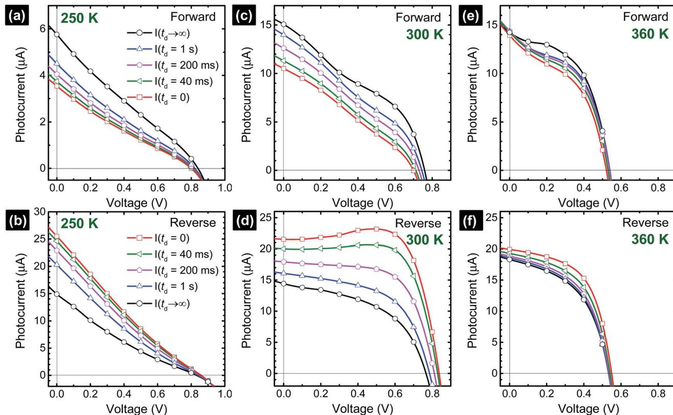
Fig. 5 Photocurrent versus voltage curves composed from the time-dependent data shown in Fig. 2 considering the different delay times ( $t_d$ ). The steady-state photocurrent values,  $I(t_d \rightarrow \infty)$ , were calculated from the semi-logarithmic plots.
