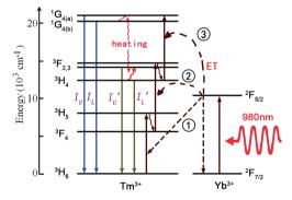
Fig. 6 The mechanism of optical thermal sensing through  $Yb^{3+}-Tm^{3+}$  energy transfer under 980 nm infrared excitation.
