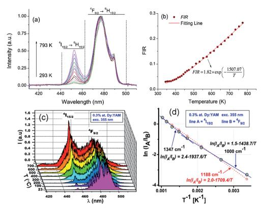
Fig. 16 Temperature dependent (a) emission spectra and (b) fluorescence intensity ratio (FIR) between the 455 nm and 478 nm emissions for the  $BaYF_5:2\%Dy^{3+}$  sample. Temperature dependent (c) emission spectra and (d) Arrhenius plot of the intensity ratio for  $Dy^{3+}$  doped  $Y_4Al_2O_9$  crystals. Reproduced from ref. 72 and 73 with permission of Optical Society of America and Elsevier.
