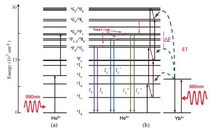
Fig. 9 The mechanism of optical thermal sensing through (a) up-conversion of the  $Ho^{3+}$  ion under 890 nm infrared excitation, and (b)  $Yb^{3+} - Ho^{3+}$  energy transfer under 980 nm infrared excitation.
