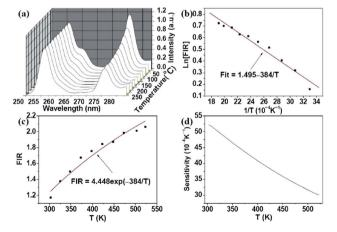
Fig. 5 Temperature dependent (a) spectrum of  $\rm Er^{3+}$  ions from  $^4D_{7/2}$  and  $^4G_{9/2}$  levels; (b) log plot of the FIR; (c) FIR relative to the temperature; and (d) sensor sensitivity under 980 nm excitation. Reprinted from ref. 38 with permission of Optical Society of America.
