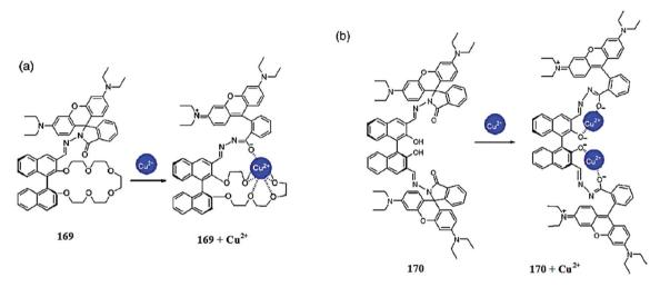
Chemical structure of receptors 169 and 170, along with the copper complexation mechanism.
