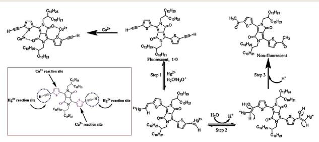
Fig. 117 Chemical structure of receptor 143 and the proposed metal sensing mechanism; inset describes the reaction site inside the receptor.
