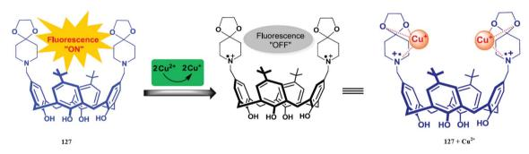
Fig. 106 Chemical structure of receptor 127 and the proposed copper complexation mechanism.
