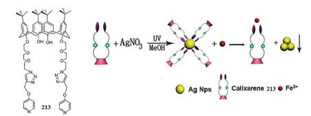
Fig. 178 Chemical structure of calix[4] arene 213, synthesis of 213-Aq NPs and schematic of Fe<sup>3+</sup>-induced 213-Aq NP aggregation.
