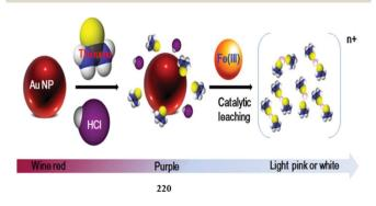
Fig. 184 Proposed mechanism for the colorimetric change of AuNPs 220 induced by Fe<sup>3+</sup> ions in the presence of an acidic thiourea system.
