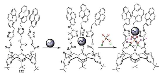
Fig. 196 Chemical structure of receptor 232 and the proposed complexation mechanism toward zinc/H<sub>2</sub>PO<sub>4</sub><sup>-</sup>.
