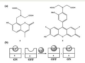
Fig. 4 Chemical structure of receptors 4 and 5 (a); schematic of a ratiometric  $Cu^{2+}$  sensing system (b).
