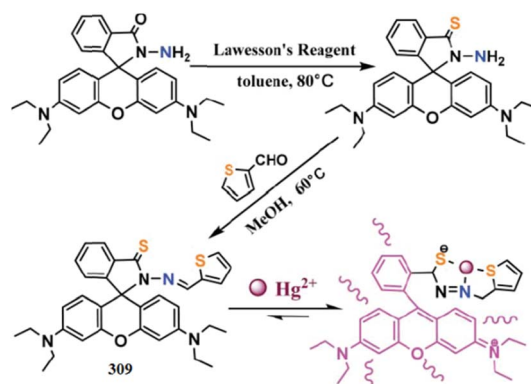
Fig. 271 Synthetic route, molecular structure and \text{Hg}^{2+} binding mode of ligand 309 .
