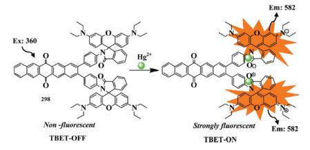
Fig. 262 Chemical structure of ligand 298, Hg<sup>2+</sup>-induced TBET-Off-On mechanism and the bioimaging response.
