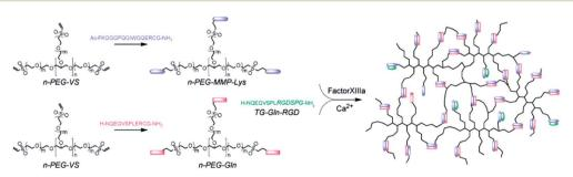
Fig. 4 Schematic of factor XIIIa-catalyzed formation of a PEG-peptide biomimetic hydrogel. Factor XIIIa was used to cross-link two PEG-peptide conjugates (*n*-PEG-MMP-Lys and *n*-PEG-Gln) in combination with a cell adhesion peptide (TG-Gln-RGD) to form multifunctional biomimetic hydrogels. Reprinted with permission from.<sup>64</sup> Copyright 2007, American Chemical Society.
