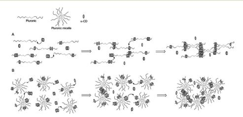
Fig. 10 Temporal gelation mechanism of linear Pluronic (e.g.: F6810 and F6820) or Pluronic micelles (e.g.: F12710) and  $\alpha$ -CD. (A) Gelation without micelle formation. (B) Gelation in the presence of micelles. Reprinted with permission from. Copyright 2013, American Chemical Society.
