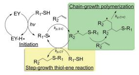
Fig. 3 Schematic of a visible light initiated mixed-mode photopolymerization for forming hydrogels (EY: eosin-Y; hv: visible light source;  $k_{p,S-C}$ ,  $k_{p,C=C}$ ,  $k_{p,CT}$ : kinetic constants for thiol–carbon radical propagation, carbon–carbon radical propagation, and chain-transfer, respectively).<sup>36</sup>
