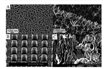
Fig. 8 Examples of plasma-treated surfaces. (A) Petal- and tree-like graphene networks. (B) Titanium pillars structured in bulk material using reactive ion etching with fluorine plasma. (C) Collagen-grafted titanium surface *via* allylamine-glow discharge treatment and collagen crosslinking. Reprinted with permission from ref. 133–135.
