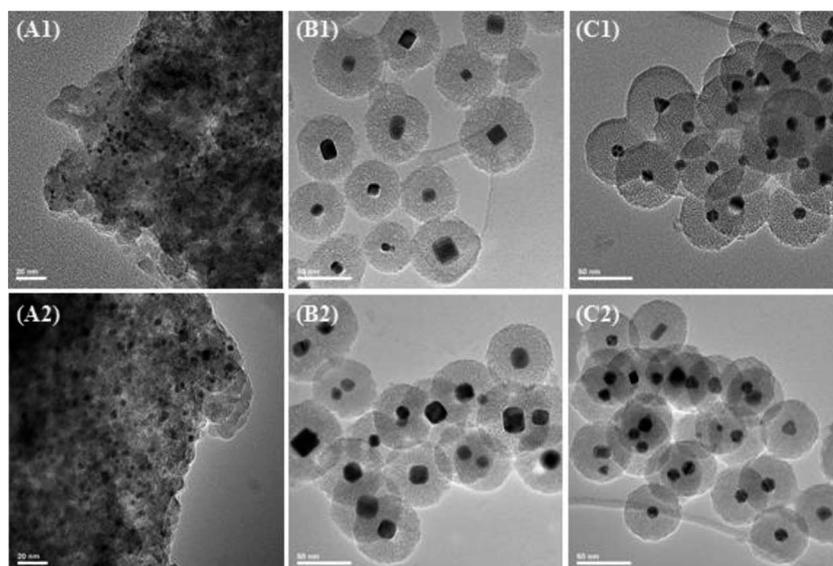
Fig. 11 TEM images of Pd<sub>imp</sub>/SiO<sub>2</sub> (A), Pd<sub>cub</sub>@SiO<sub>2</sub> (B) and Pd<sub>pol</sub>@SiO<sub>2</sub> (C) catalysts before (1) and after (2) catalytic test. Reproduced from ref. 128 Copyright (2015), with permission from Elsevier.
