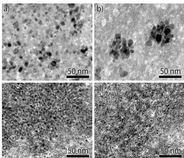
Fig. 7 Bright-field TEM images of Ni/SiO<sub>2</sub> catalysts with different Ni particle sizes after reduction: (a) ~8 nm, (b) ~9 nm, (c) ~4 nm, and (d) ~3 nm. Reproduced with permission from ref. 66 Copyright (c) [2014 WILEY-VCH Verlag GmbH & Co. KGaA, Weinheim].
