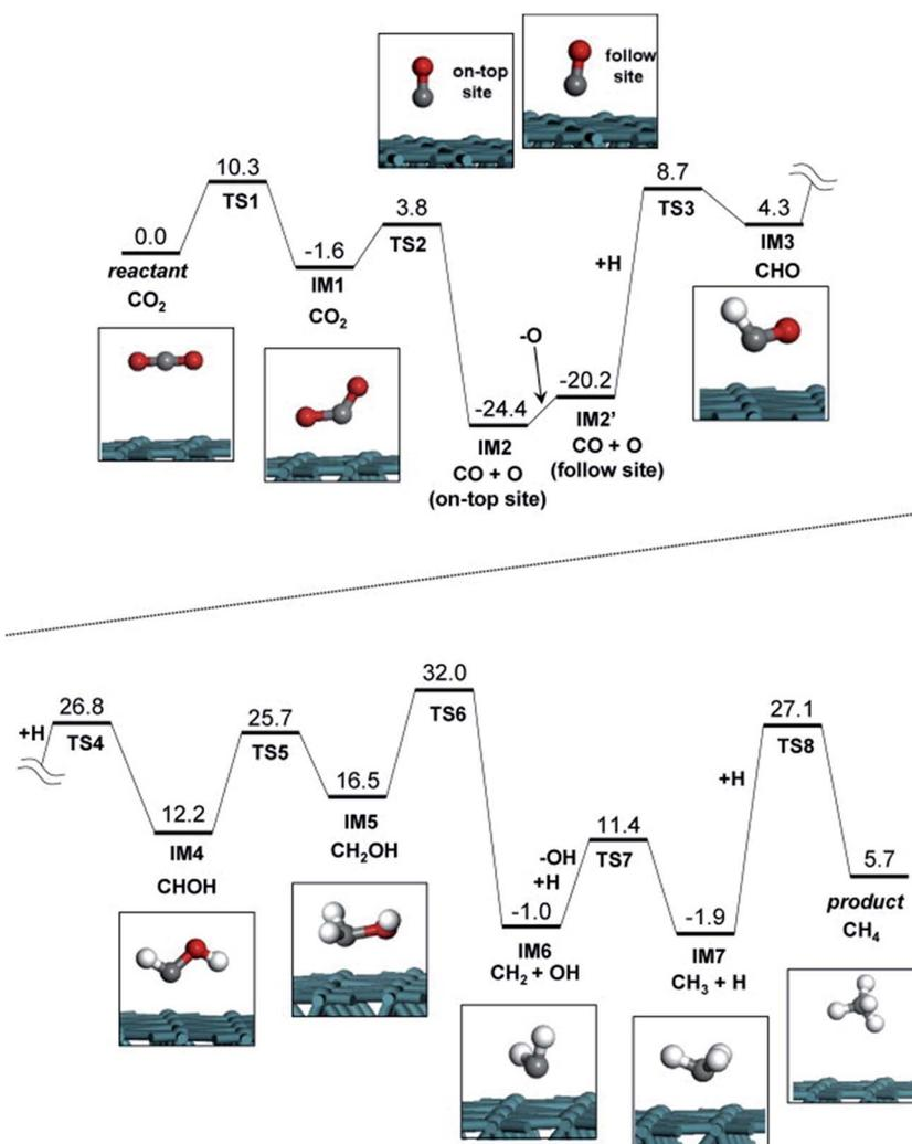
**Fig. 12** Potential energy diagram for carbon dioxide methanation on the Ru surface slab structure. Each reactant, product and intermediate structures are also shown in the inset of the figure. Reproduced with permission from ref. 224 Copyright (2014), with permission from Elsevier.
