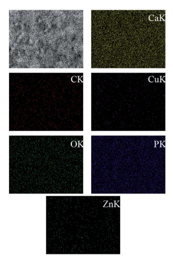
Fig. 4 EDS mapping of the lateral distribution of Zn, Cu, Ca, P, and O compared to the SEM image of the same area for ZnCuHAP coating.
