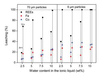
Fig. 7 Leaching (%) of Co, Fe and REEs (Nd + Dy) from two different milled roasted NdFeB magnets (≈70 μm and 6 μm). The leaching is shown as function of time (24 and 72 h) and as function of the water content in the ionic liquid (2.5, 5, 7.5 and 10 wt%). The solutions were stirred 600 rpm at 90 °C.
