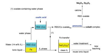
Fig. 19 Overview of the proposed stripping process based on oxalic acid precipitation of REE(III) and Co(II) ions and phase transfer of iron(III) as a water-soluble oxalate complex. This process allows full recovery of the ionic liquid. The cobalt can be removed by treating the mixed REE/Co oxalate precipitate with aqueous ammonia.
