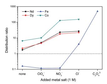
Fig. 11 Influence of added metal salts (1 M) with varying anions on the distribution ratio of Nd(III), Dy(III), Fe(III) and Co(III) ions in a biphasic [Hbet]– $[Tf_2N]-H_2O$  system. A high distribution ratio corresponds to a greater affinity for the water phase. Oxalate forms highly insoluble complexes with REE(III) and Co(II) ions.
