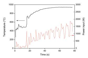
Fig. 3 Heating of demagnetized NdFeB magnet particles ( $\approx$ 400 µm) with a monomodal high-temperature microwave set-up. The temperature was raised in two steps: first it was stabilized at 500 °C and then at 950 °C. The power input (W) and temperature (°C) are shown *versus* time (s). The temperature range under 250 °C was not accessible with the infra-red temperature probe.
