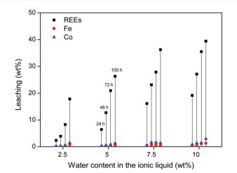
Fig. 4 Leaching (%) of Co, Fe and REEs (Nd + Dy) from large roasted NdFeB particles ( $\approx\!300~\mu m$ ). The leaching is shown as function of time (24, 48, 72 and 100 h) and as function of the water content in the ionic liquid (2.5, 5, 7.5 and 10 wt%). The solutions were stirred at 600 rpm and 90 °C.
