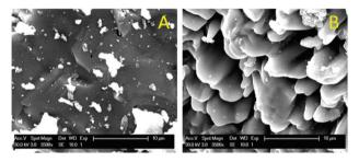
Fig. 6 SEM images (magnified 3500x) of the surface of the particles before (A) and after (B) leaching.
