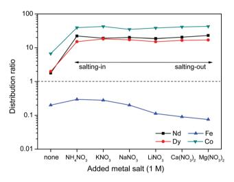
Fig. 14 Influence of added metal salts (1 M) with varying cations on the distribution ratio of Nd(III), Dy(III), Fe(III) and Co(III) ions in a biphasic [Hbet]-[Tf<sub>2</sub>N]-H<sub>2</sub>O system. A high distribution ratio corresponds to a greater affinity for the water phase.
