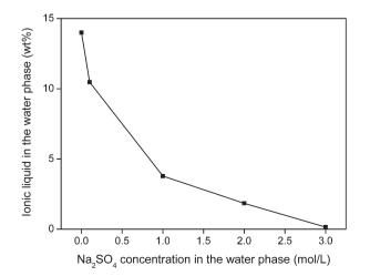
Fig. 20 Salting-out of ionic liquid from water using  $Na_2SO_4$ . This way, loss of ionic liquid can be avoided.
