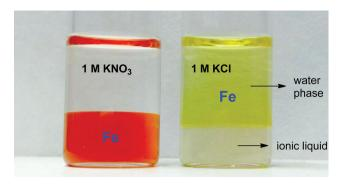
Fig. 12 Reversal of iron( $\parallel$ ) distribution when adding a non-coordinating salt (KNO<sub>3</sub>) compared to a salt with coordinating anions (KCl). The upper and lower phase consist of water and [Hbet][Tf<sub>2</sub>N], respectively.
