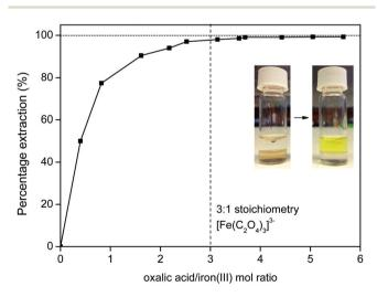
Fig. 18 Stripping of iron(III) from the ionic liquid to the water phase using oxalic acid. The oxalic acid regenerates the ionic liquid and transfers the iron(III) ions to the water phase as the highly soluble  $\text{Fe}(C_2O_4)_3^{3-}$  complex. The photograph shows the transfer of iron from the ionic liquid phase (left) to the water phase (right).
