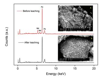
Fig. 5 SEM images (magnified 250x) and EDX spectrum of the surface of the large NdFeB particles (≈300 µm) before (A) and after (B) leaching.
